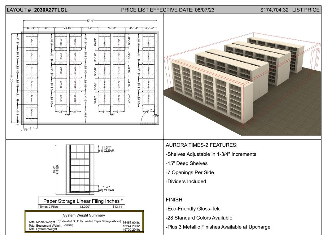
\* Designed For A 9' Ceiling Allowing 18" For Sprinkler Clearance
